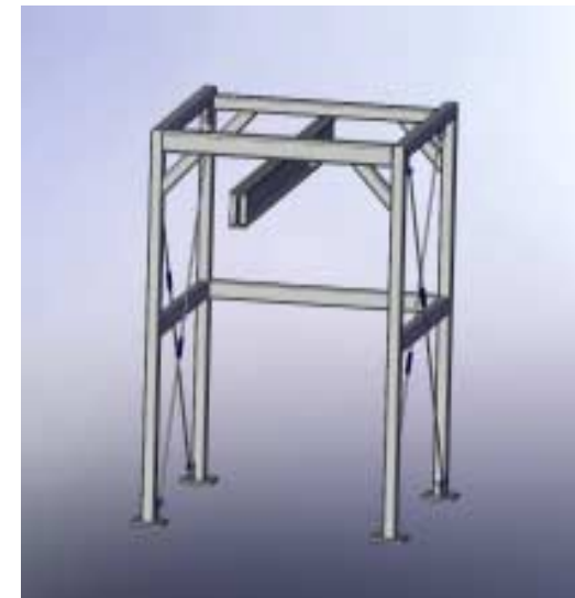
Upper frame support for big-bag-setting with crane
