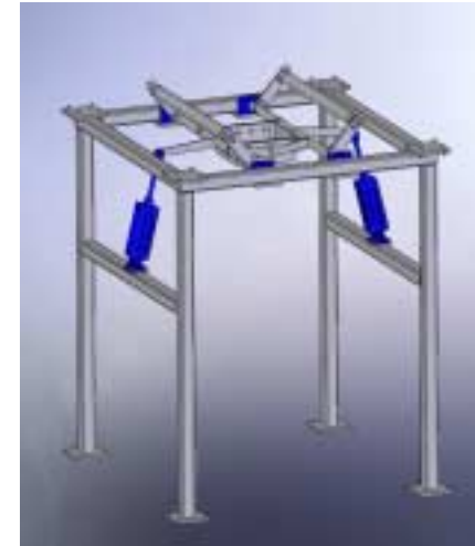
Lower frame support with double-rocker and tumble-frame as a discharge aid
