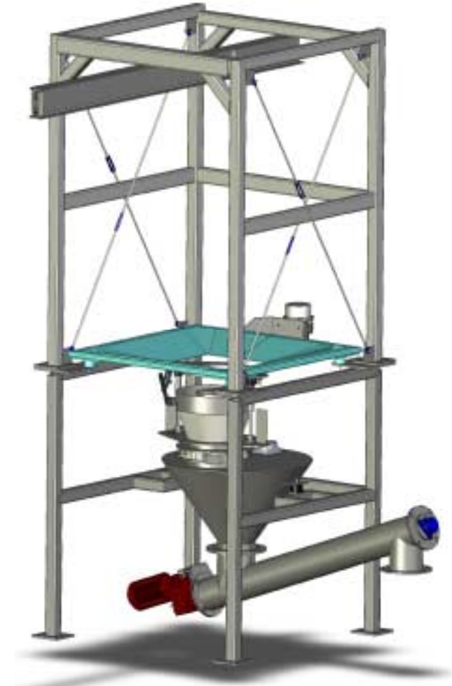
Example: with vibration hopper, dust-tight docking, , valve, storage hopper, metering feed screw
