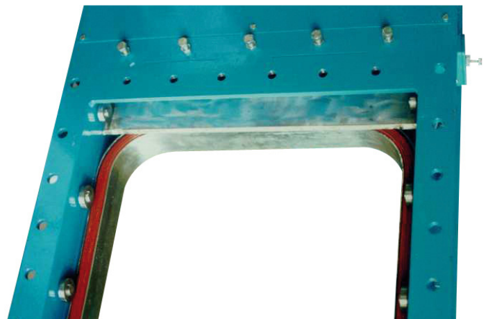
Detail: pneumatically inflatable sealing
